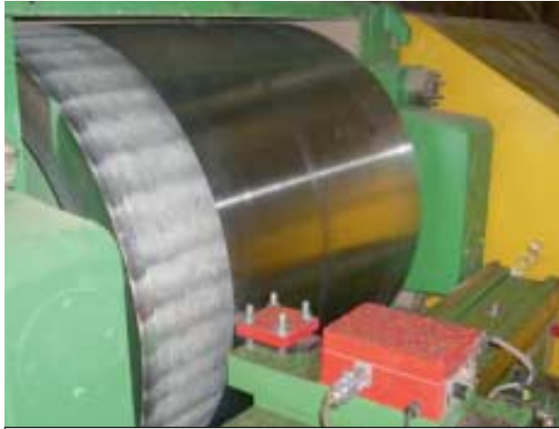
»3 With the Twin roller turning machine, the turning time can be halved
