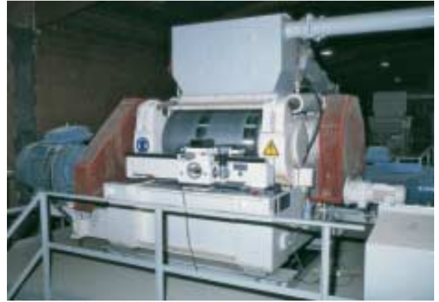
»3 With the Twin roller turning machine, the turning time can be halved
